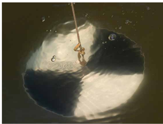
Figure 3.2. Water clarity is often measured using a secchi disk.
