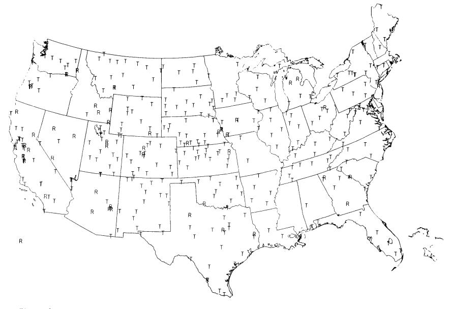
Figure 1--Distribution of Class A pan stations which make concurrent measurements for computing FWS evaporation by equation 3. Stations identified by an R were not equipped with sensors to record additional data until the latter part of the 1956-70 time base.
