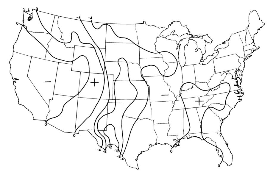
Figure 7--Deviation in inches of May-October free water surface evaporation  $E_{mf}$  (computed using meteorological factors) from equivalent map points  $E_{m2}$  (station point values from map 2) derived from the analysis of observed values. Map value =  $E_{mf} - E_{m2}$
