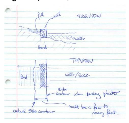
The only way to remedy this is by doing a proper contour survey. A couple of those lines exist on the buy-down maps, a 2462 and a 2466 contour line.
