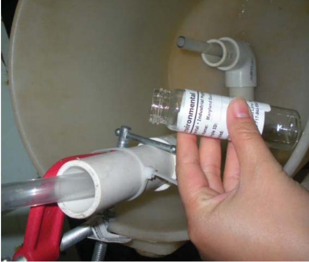
Figure 8. Inverted bottle technique for dissolved-methane collection of well-water samples. Step A: Clear tubing is connected to untreated water source (e.g., pressure tank spigot), and the water is turned on to fill up the sampling bucket. Step B: Cap is removed from glass vial. Step C: Glass vial is inverted and placed over the clear tubing. Water fills the vial and is allowed to flush three vial volumes before the vial is capped underwater (modified from Hirsche and Mayer, 2009).
