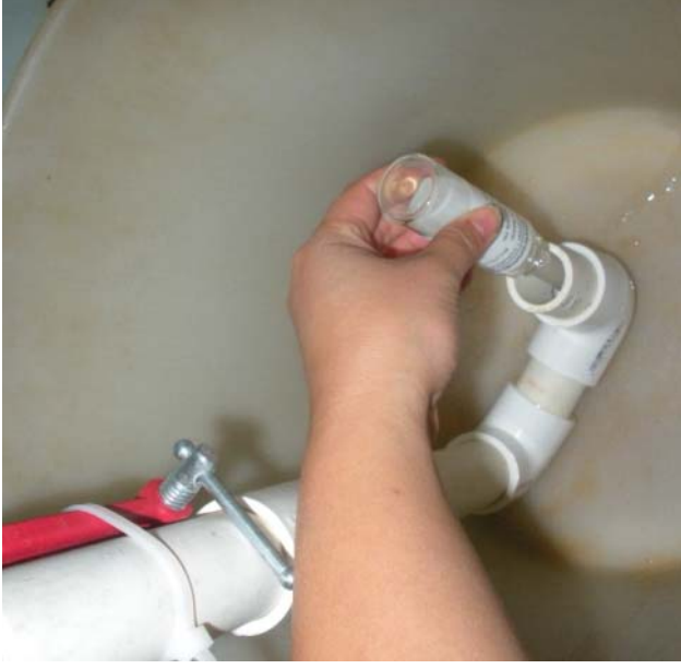
Figure 8. Inverted bottle technique for dissolved-methane collection of well-water samples. Step A: Clear tubing is connected to untreated water source (e.g., pressure tank spigot), and the water is turned on to fill up the sampling bucket. Step B: Cap is removed from glass vial. Step C: Glass vial is inverted and placed over the clear tubing. Water fills the vial and is allowed to flush three vial volumes before the vial is capped underwater (modified from Hirsche and Mayer, 2009).
