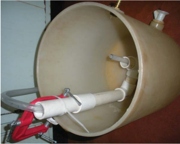
Figure 8. Inverted bottle technique for dissolved-methane collection of well-water samples. Step A: Clear tubing is connected to untreated water source (e.g., pressure tank spigot), and the water is turned on to fill up the sampling bucket. Step B: Cap is removed from glass vial. Step C: Glass vial is inverted and placed over the clear tubing. Water fills the vial and is allowed to flush three vial volumes before the vial is capped underwater (modified from Hirsche and Mayer, 2009).
